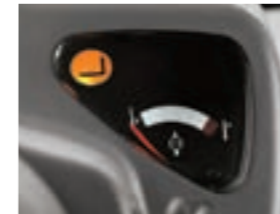
The interlock state is also indicated on the meter panel.
